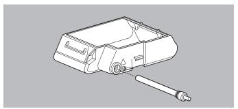
1. Unscrew the element from the base of the humidifier.
