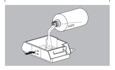
5. Fill the base of the humidifier with fresh, cold water up to the mark (max. 400 ml).
