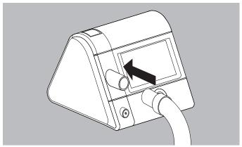
1. Connect the respiration hose to the device outlet.
