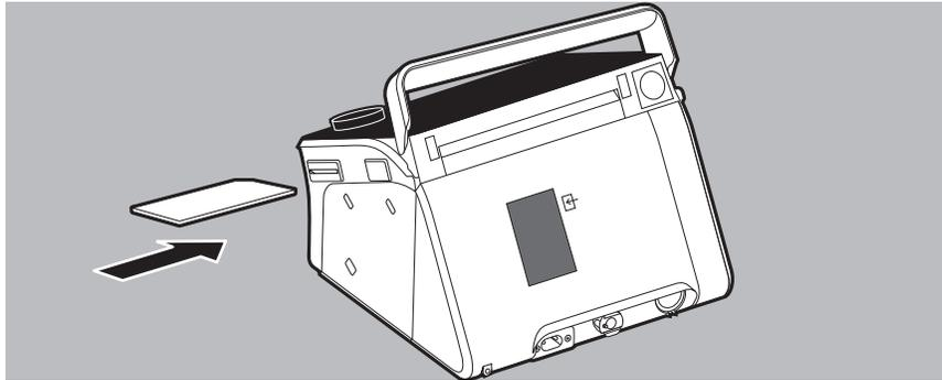
1. Push the SD card into the SD card slot until you hear it engage. The SD card symbol
