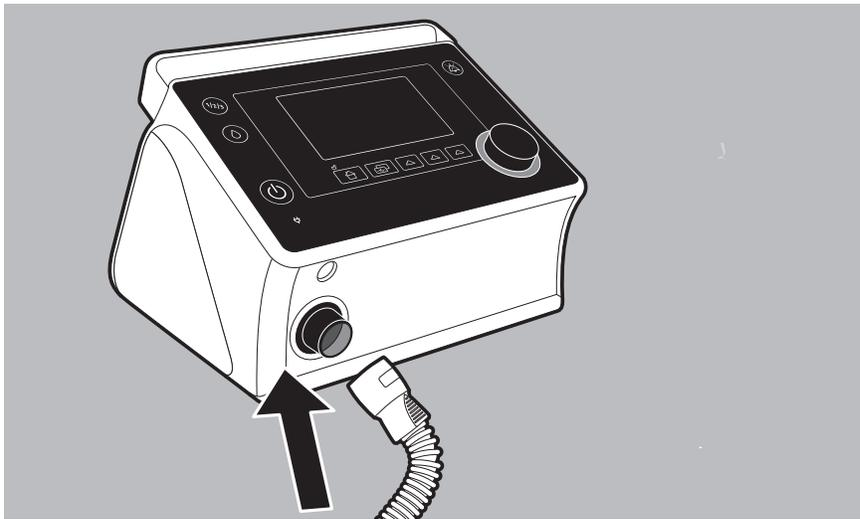
1. Push breathing tube onto the device outlet port.
