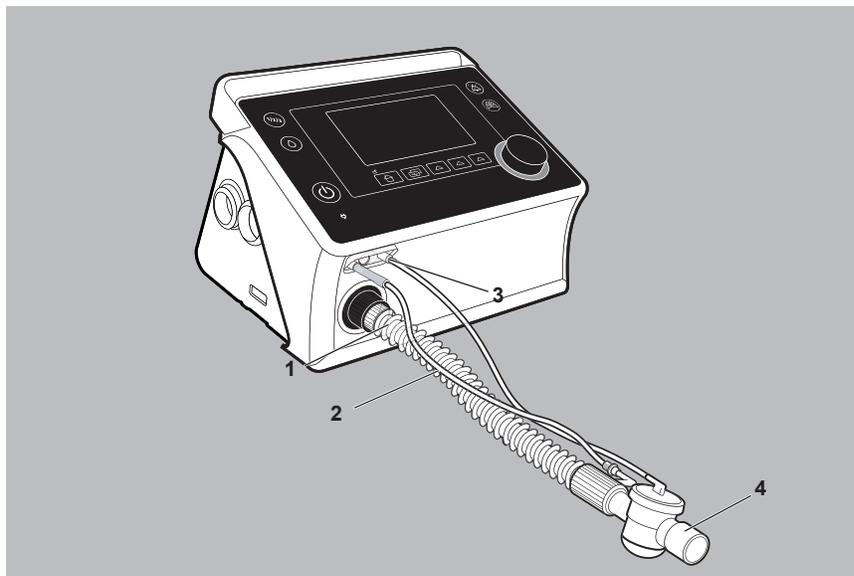
1. Push the free end of breathing tube **1** onto the device outlet port.
